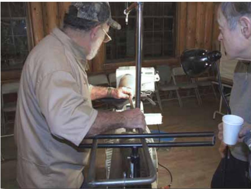
The key to getting it right: the cutting edge of the hollowing tool must be at exact lathe center and the entire tool setup must be parallel to the lathe bed. Jerry makes it look pretty simple and with the appropriate tools and setup there's much more control when hanging that far over the tool rest. The laser beam guide provides great feedback for wall thickness.
