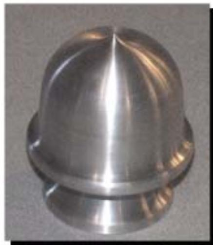
*During last months metal spinning class Terry Tynan, the instructor, demonstrated spinning techniques using mandrels of various designs. This acorn project was spun on two separate forms, one consisting of what's called a plug mandrel. Made in two pieces at the waist of the form it allows spinning reentrant shapes such as the base of the acorn.*
