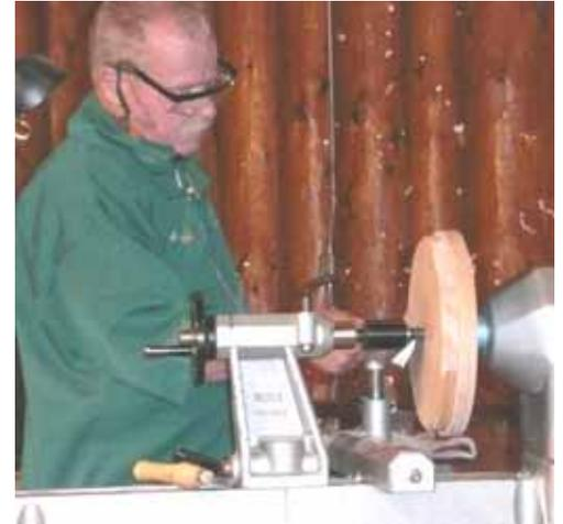
*Figure 2. Turning away the square corners with a bowl gouge.*
