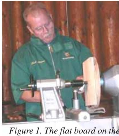
*Figure 1. The flat board on the lathe between the faceplate mounted disk and the live tail center.*
