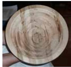
Figure 8. The glued up blank ready to turn.
