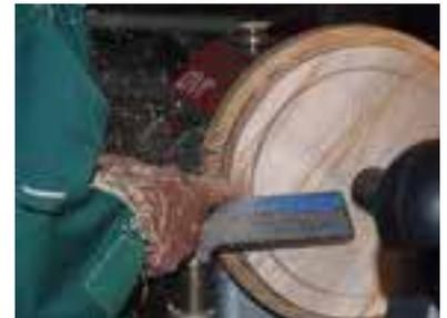
*Figure 3. Cutting the first ring loose.*
