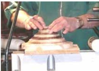
Figure 6. Applying the final piece to the stack of rings before clamping
